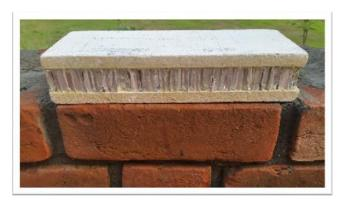
As to maintenance? There is hardly any! Since we use honeycomb aluminum and magnesium oxide (MGO) sandwich panels our structures do not contain any sand, cement, steel, mortar or bricks, therefore there is no plaster that will chip or crack. A fresh overcoat of paint every few years does the trick. If the exterior MGO surface is cladded, it is nearly indestructible.
